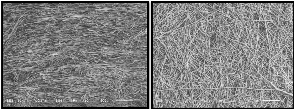
**SoftSeal-STF structure using scanning electron microscopy (SEM at 30X). Discrete and small fibers can be seen on edge view (left) and top of pad (right).**
