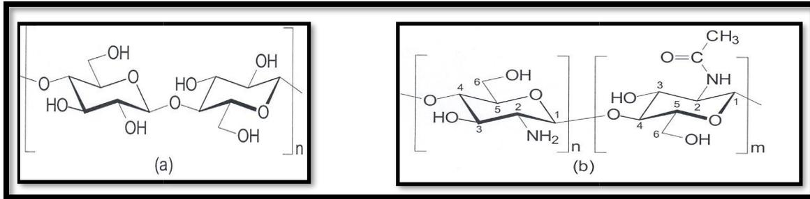
**Chemical structures of Cellulose (left) and Chitin – Chitosan (right)**
